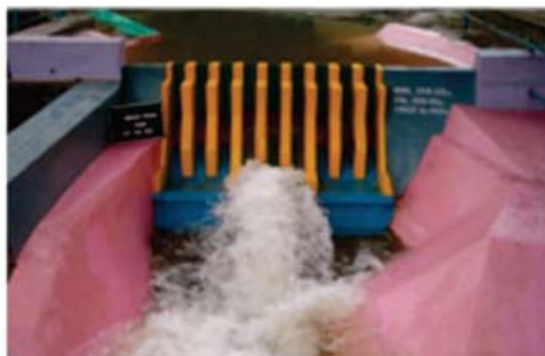
Photo 4 : Spray generation and subsequent failure of bank in Salal project
