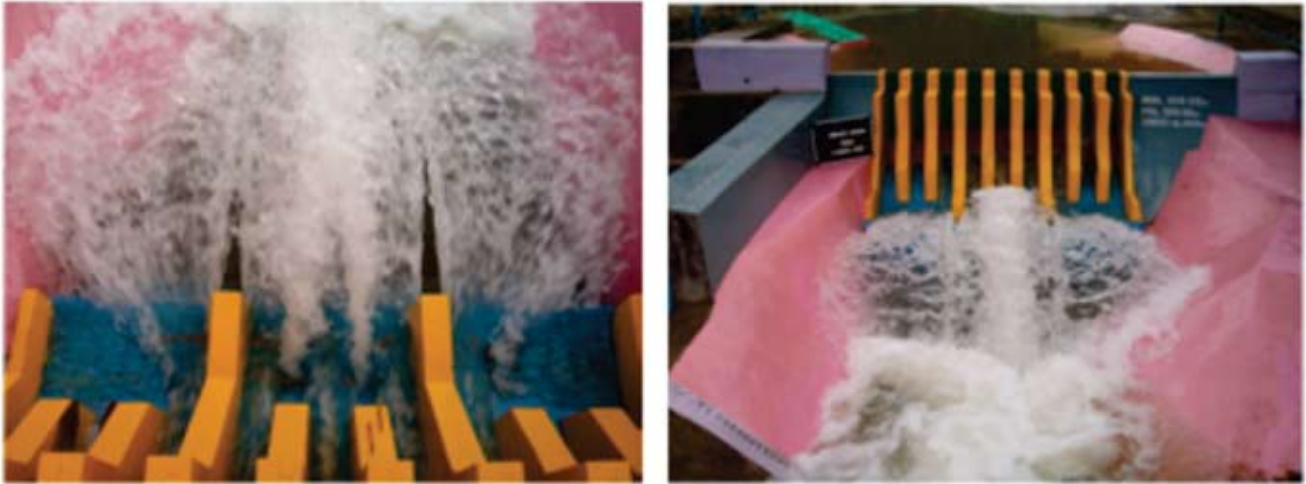
Photo 5: Spillway Operation with divide walls up to lip
