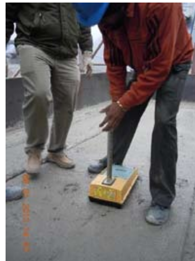
Fig. 18 : Nuclear densimeter in use
