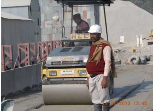
Fig. 12 : 2.5 MT vibratory roller under operation
